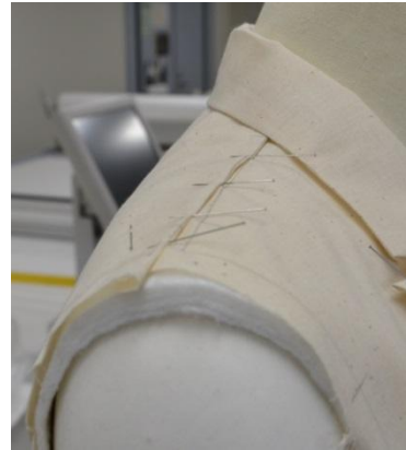
Figure 6 Modifications of shoulder parts using fitting patterns
