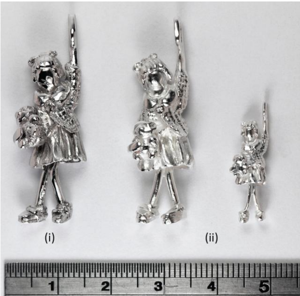
Figure 22 – “Sofia” pendant: (i) traditional production process, (ii) new production process with digital technology
