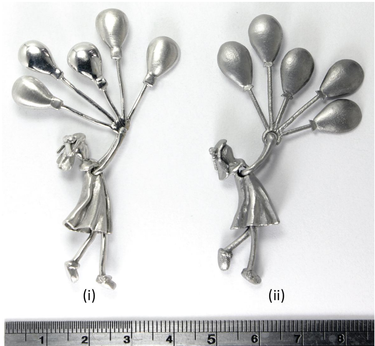
Figure 24 – “Beatriz and the Balloons” Pendant: (i) traditional production process, (ii) new production process with digital technology
