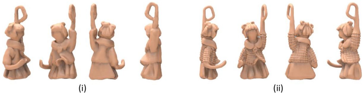
Figure 13 – Modifications done by digital sculpture in a three-dimensional model digitalized by Structured-Light: (i) digitalized model; (ii) modified model.
