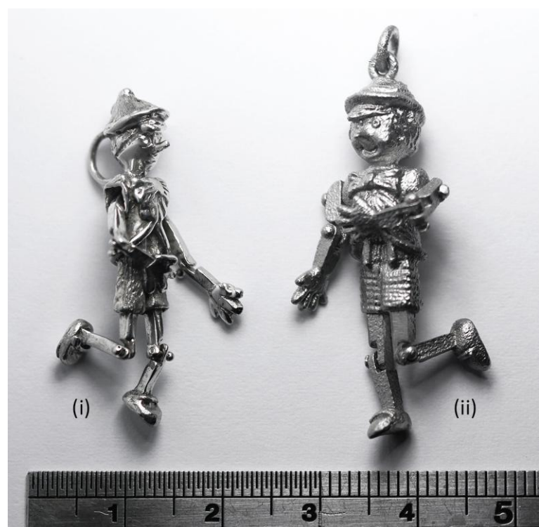
Figure 25 – “Pinocchio” Pendant: (i) traditional production process, (ii) new production process with digital technology
