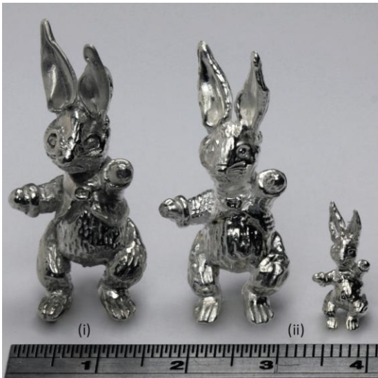
Figure 21 – “Alice’s Rabbit” pendant: (i) traditional production process, (ii) new production process with digital technology
