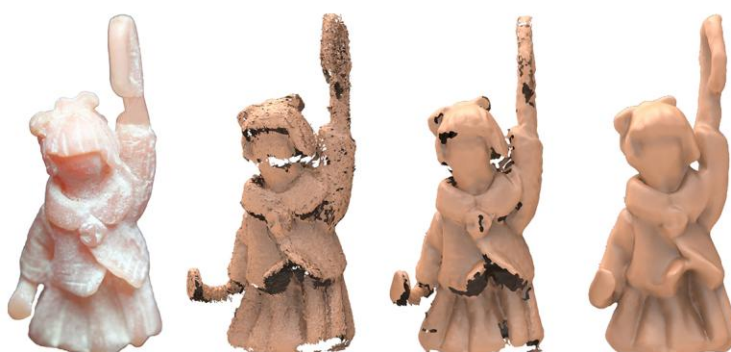
Figure 7 – Company's wax model digitalized by Structured-Light and sequence of digitalization treatment.
