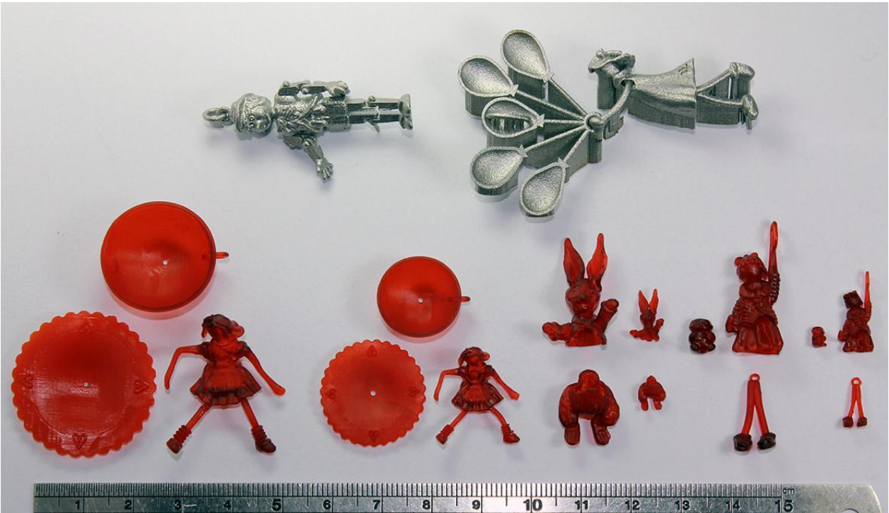
Figure 18 – Models printed in Direct Metal Laser Sintering and Digital-Light Processing
