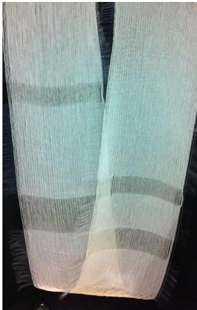
Figure 8: Photonic fabric produced by plain weave.
