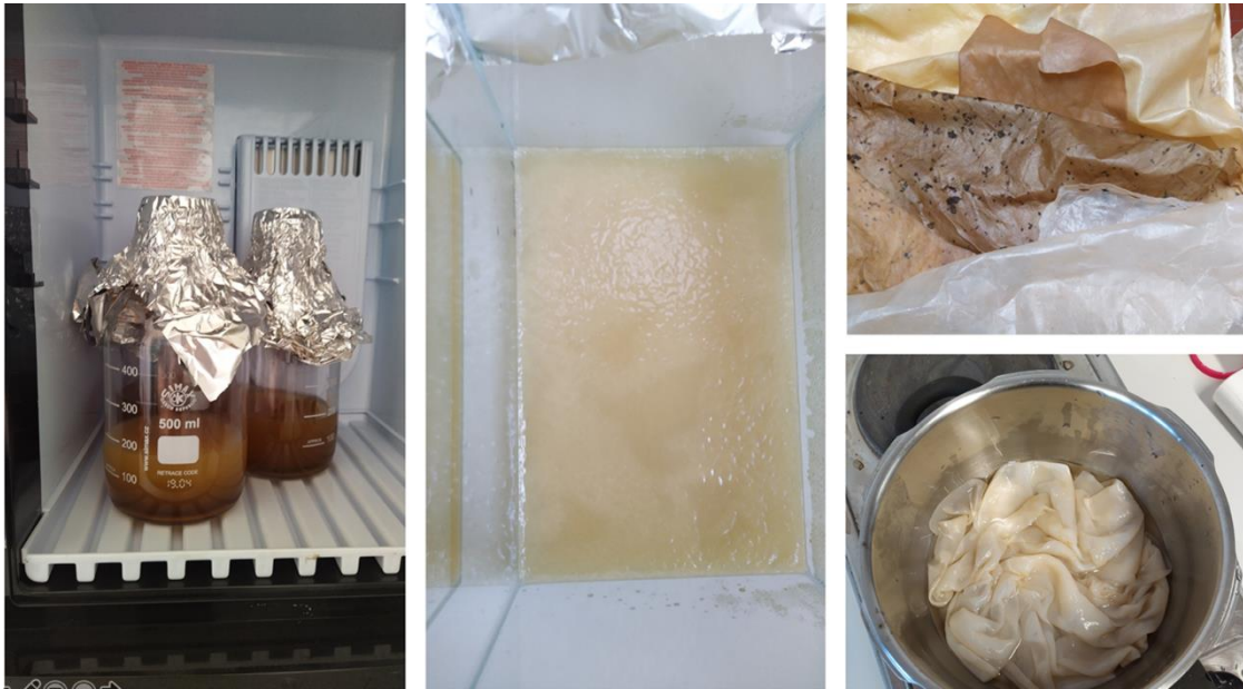
Figure 6: lab collage: K.Xylinus cultures in the incubator, grown BC pellicle in glass broth, BC fabric quality samples after post processing (left to right, up to down)
